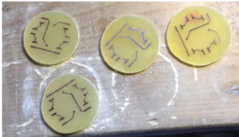
Figure 29. Cutting out PCB board.
