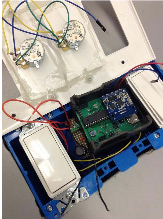
Figure 17. Light switches and dimmers attached to microcontroller.
