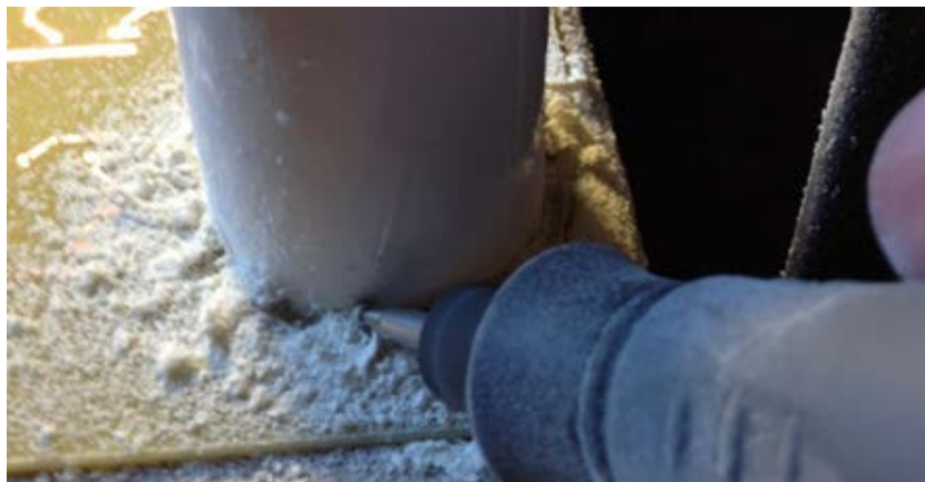
Figure 29. Cutting out PCB board.
